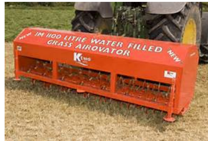
Spiker with water tank for extra weight
