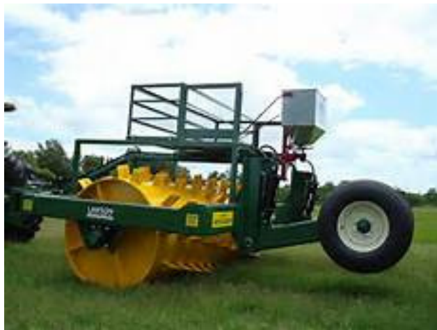
Roller spiker with grass seeder and frame for extra weight
