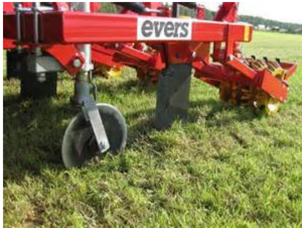
Pre-cutting Disc and Closer leg spacing
