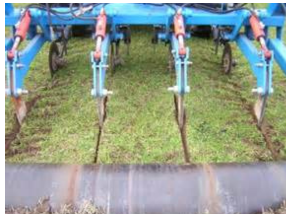
Roller for depth control and break back legs to reduce bringing stones to the surface
